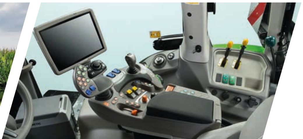
> Ergonomic joystick MaxCom with lift buttons, engine/transmission commands, button for managing turns at the headland and two proportional hydraulic distributors.
